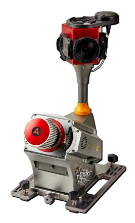
Whatever the task is, the Alpha3D is easily mounted on a variety of platforms, including different type of vehicles, trains, railway trolleys and boats, rapidly and efficiently collects the high density, accurate point clouds and powerful images data but also adds extra information from additional sensors, such as high-resolution camera, thermal camera, echo sounder or extra profiler.
